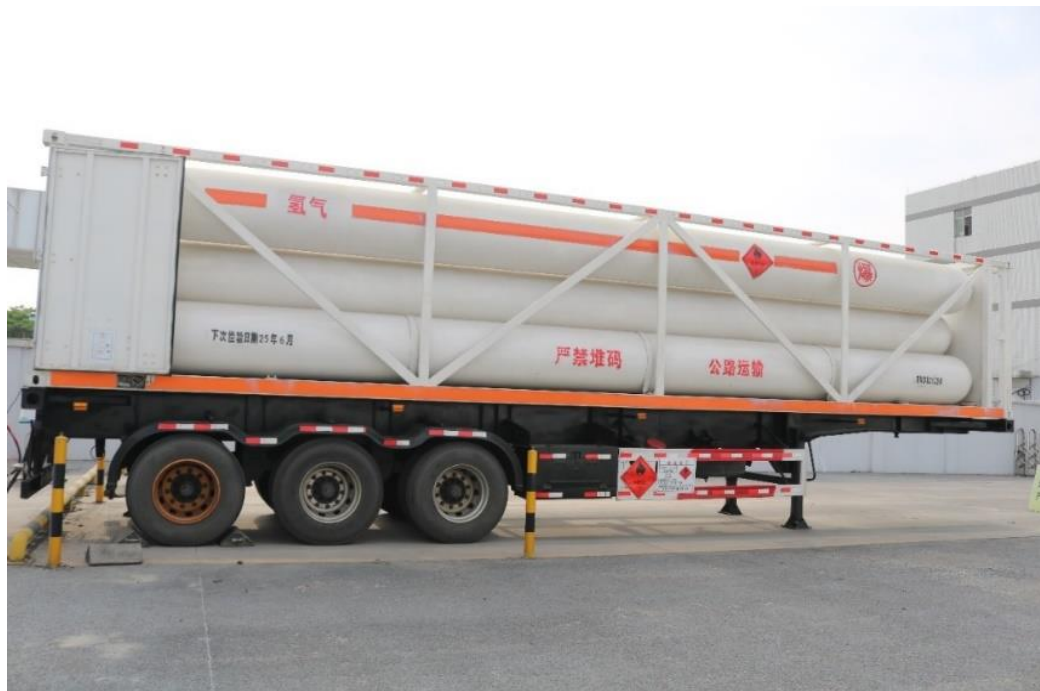
Pressure receptacles on tube trailer
