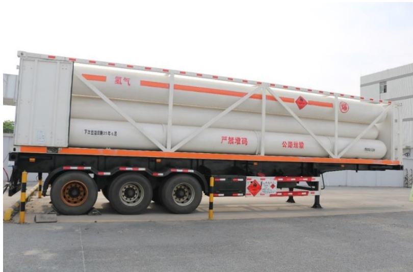
Pressure receptacles on tube trailer
