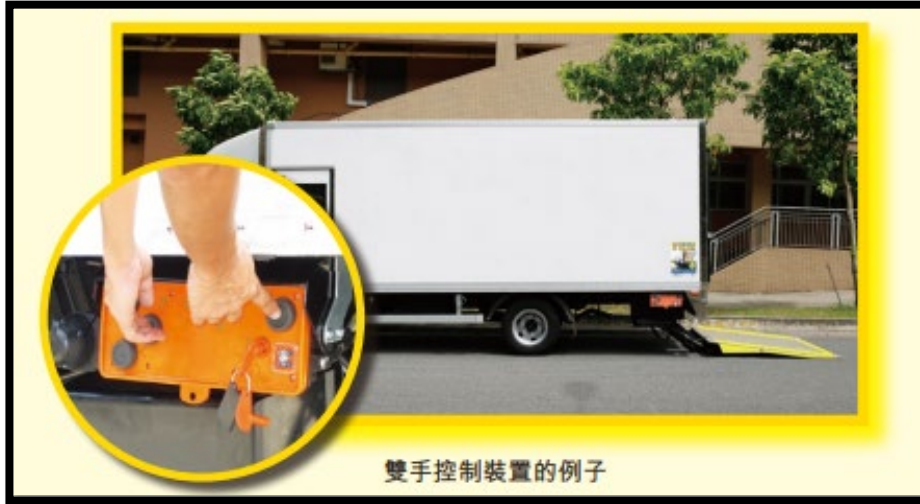
Two-hand control device
